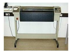
Plotters use ink and fine pens held in carriage to draw very detailed designs on paper. They are used for construction plans, engineering drawings and other technical illustrations. Nowadays traditional plotters are being replaced with wide-format inkjets.
