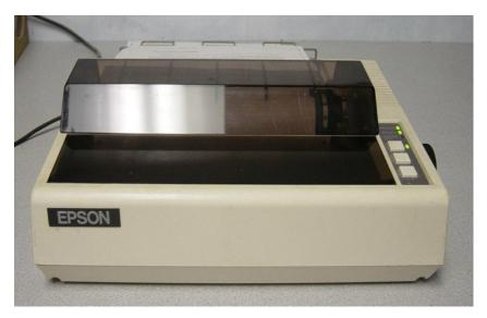
**Dot-matrix printers** الطابعات النقطية : use pins to print the dots required to shape a character. They can print text and graphics, however, they produce relatively low resolution output-72 to 180 dots per inch (dpi). They are used to print multi-part forms, self-coping paper and continuous-form labels علامات بطبعة مستمرة.
