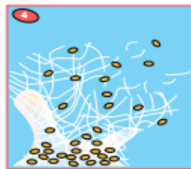
Particles of biofilm break off and the pathogens spread through the water pipe.
